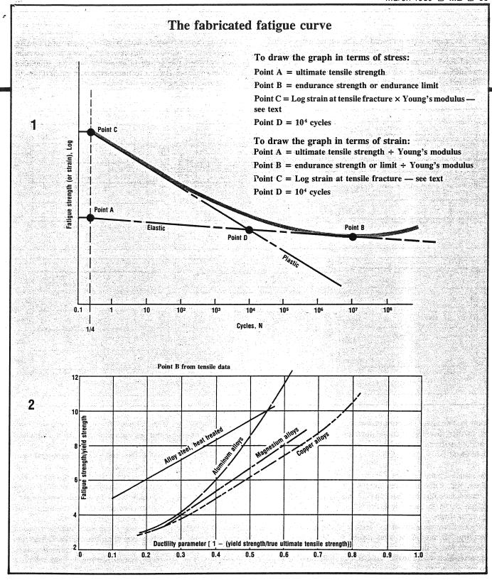
yield strength and true ultimate tensile strength for the material. Simply calculate the "ductility parameter" from handbook tensile data using the equation on the horizontal axis of the graph. Then find the "endurance-to-yield" strength ratio for the appropriate material. Multiply this ratio by "yield strength" to find the endurance value, which is Point B.
